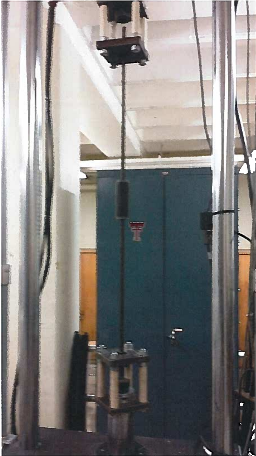
Figure 2. Fatigue Test Assembly Mounted in MTS
