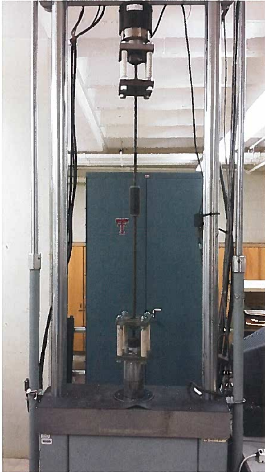
Figure 3. Static Test Assembly Mounted in MTS
